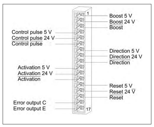
Fig. 2: 17-pole Phoenix Combicon connector MC 1,5/20-G-3,5
