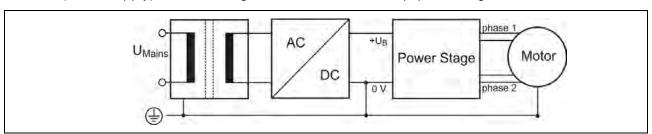
Fig. 12:PELV - Grounding: 0 V and Motor
