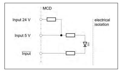
Fig. 22: Input wiring diagram
