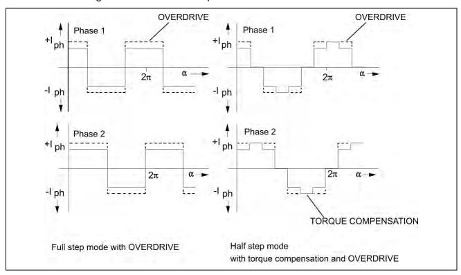
Fig. 35: Phase currents with Overdrive
