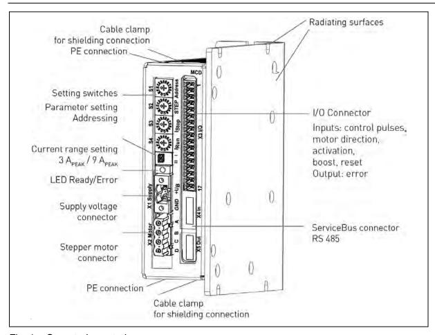
Fig. 1: Operator's controls
