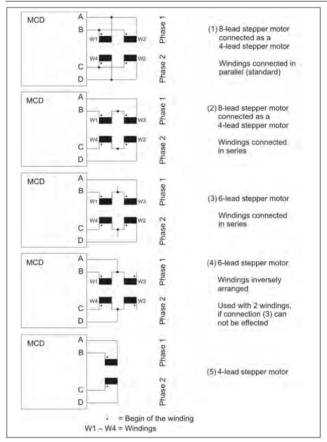
Fig. 21: Connection diagrams for 4-, 6- and 8-wire stepper motors
