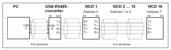
Fig. 28: Connection PC → MCD by USB-RS485-converter
