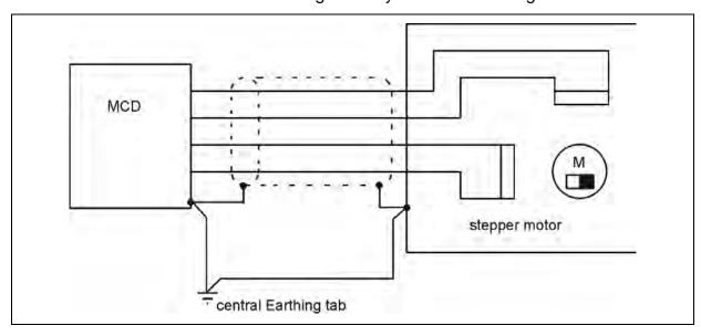
Fig. 20: Motor lead shielding
