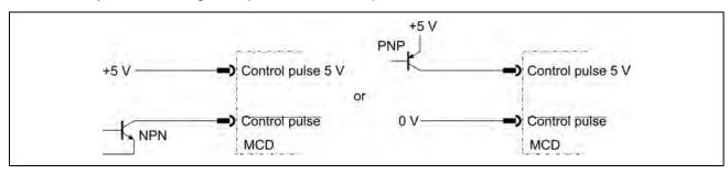
Fig. 24: Open Collector Controlling
