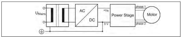
Fig. 14:PELV - Grounding: 0 V
