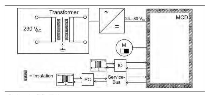
Fig. 18: Insulation MCD
