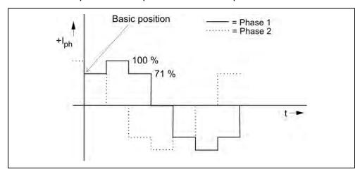
Fig. 26: Motor phases in basic position (half step)
