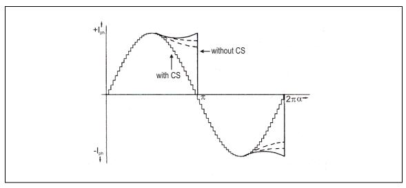
Fig. 37: Current Shaping CS
