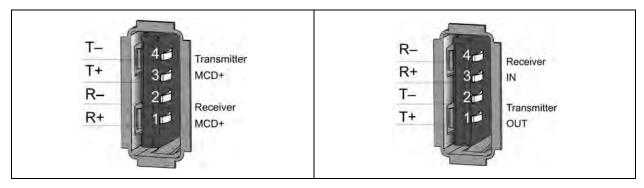
Fig. 3: 4-pole ServiceBus connector IN: X4 (DIN IEC 61076-3-107)
