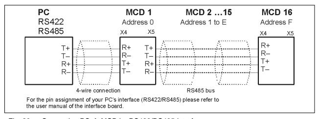
Fig. 29: Connection PC → MCD by RS422/RS485-interface
