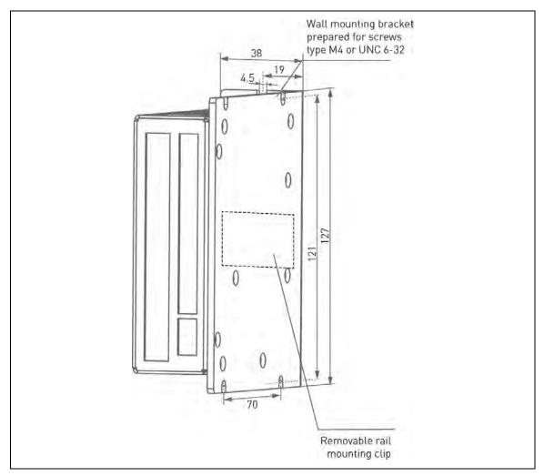
Fig. 15: Dimension in mm
