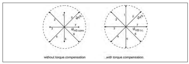
Fig. 32: Holding torques without/with torque compensation
