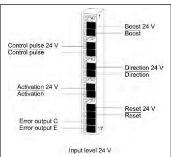
Fig. 25: Input level 5 V or 24 V connection
