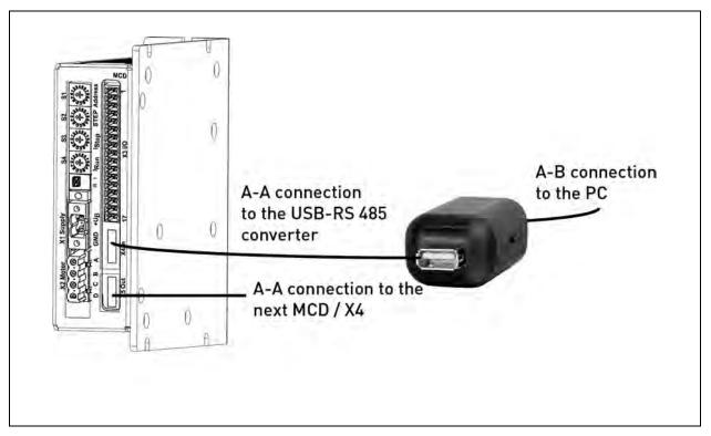
Fig. 30: Power stage MCD with phytron USB-RS485-converter
