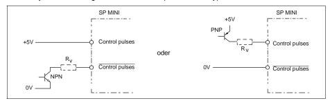
Fig. 18: Open collector controlling
