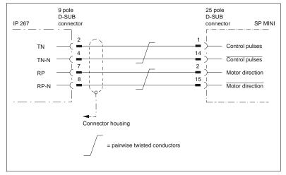
Fig. 5: Cable connections IP 267 - SP MINI
