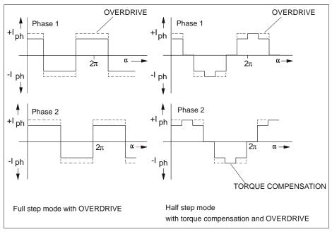
Fig. 14: Schematic curves of the phase currents with OVERDRIVE
