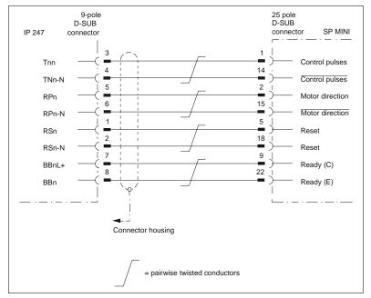
Fig. 6: Cable connections IP 247 – SP MINI 10
