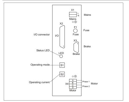
Fig. 22: Connection and display panel
