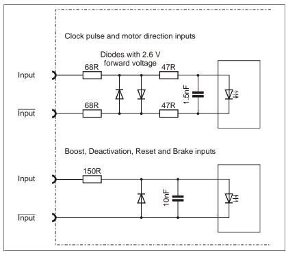
Fig. 19: Input wiring diagram for +5V logic voltage
