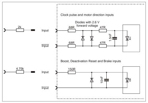
For 24 V input level connect external protective resistors to the input.
