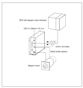
Fig. 2: SPS - SP MINI - Stepper motor
