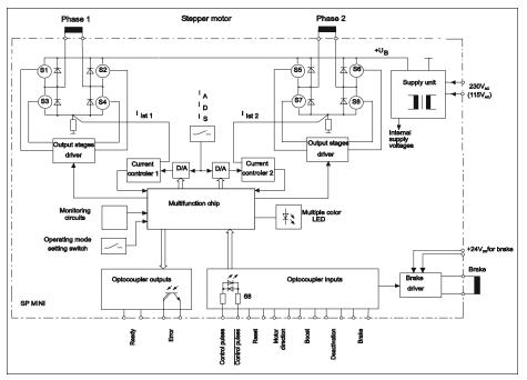
Fig. 9: Block diagram
