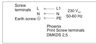
Fig. 8: Mains connection 230 V<sub>AC</sub>
