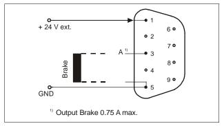
Fig. 16: Connector X3 motor brake
