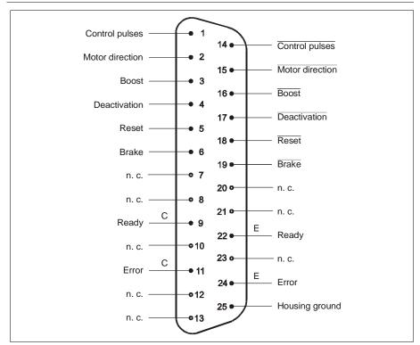
Fig. 4: 25-pole D-SUB connector according to DIN 41652
