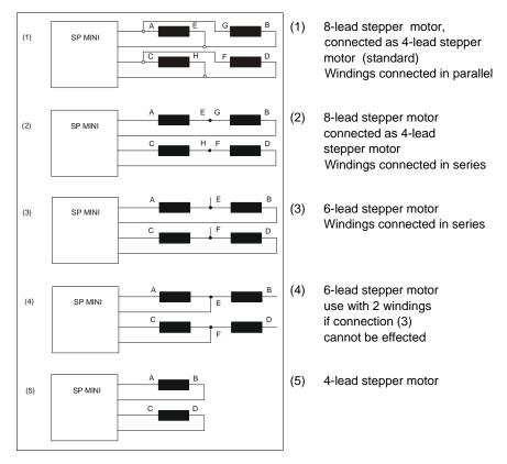
Fig. 15: Motor connection
