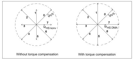
Fig. 11: Holding torques without/with torque compensation
