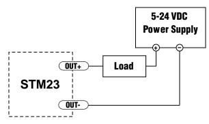
Connecting a Sinking Output
