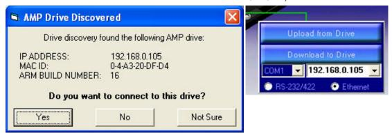
You don't need a special "crossover cable"; the drive will automatically detect the direct connection and make
