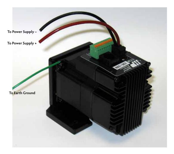
Be careful not to reverse the wires. Reverse connection may open the internal fuse on your driver and void your warranty.
