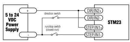
Using Mechanical Switches
