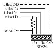
RS-422/485 4-wire "Point to Point" Wiring
